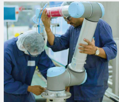
↑ A Universal Robots UR10 cobot palletizing product at L'Oréal India. ↓
